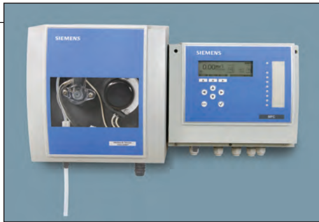
FIGURE 2. The Siemens Micro/2000 measurement module measures free and total chlorine residual, chlorine dioxide, ozone or potassium permanganate residuals in potable water, primary or secondary treated wastewater or cooling water
